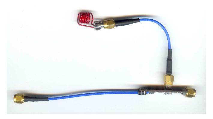
On this picture, we can see the «parallel» accessory, connected to an helical air coil inductor for measuring.
