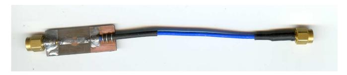
To calibrate, we use a 51 ohms resistor (smd 1206 or 0805) as reference load. For the short circuit, we used a very small sheet of copper. The small gap on the PC board trace is equivalent to a 0.051pF capacitor; this capacitor is automatically removed with the process of calibration (it does not matter its value).
