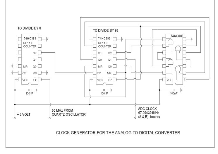
The analog to digital converters (ADS1251) need a clock. The frequency of the clock is 384 \* measurement frequency. We start with the 50MHz oscillator : 5000000=8\*93\*384\*25.0016001\*7 8\*93= frequency divider 25.0016001\*7 = number of measurements per second 384 = needed by the ADS1251 The frequency of the ADC CLOCK is 5000000/(8\*93)=67204.3 Hz
