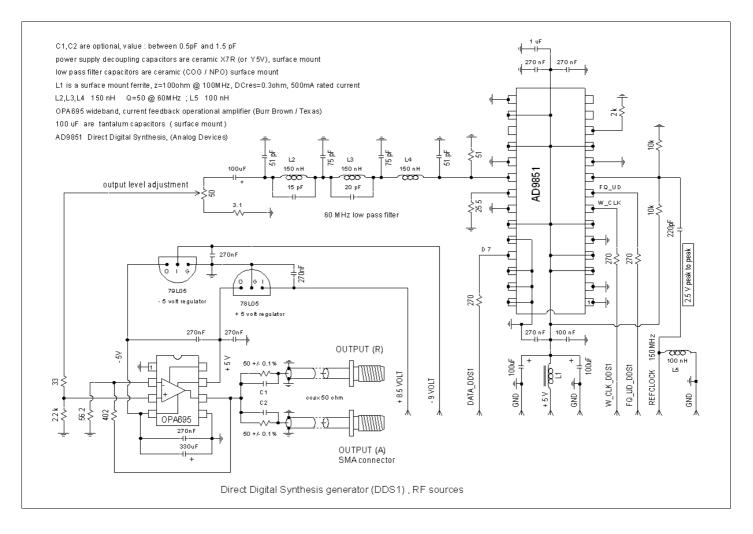
The AD9851 is the direct digital synthesis generator (Analog Devices), see the data sheet of this circuit to see how it works.
