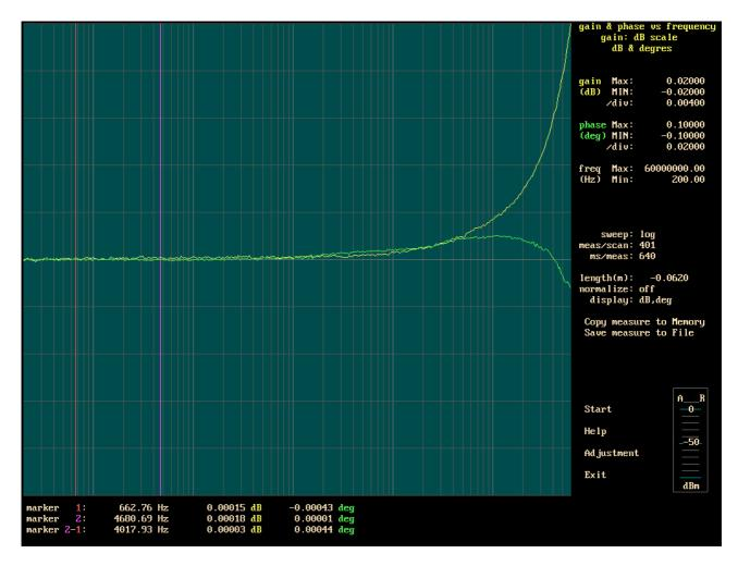
On this picture, we can see the **gain differences between the (A) channel and the (R) channel**; (without normalization, but with the "length correction " and with the " non frequency dependant " correction ). If, in the frequency range of a measurement, these gain differences are acceptable, then it is not necessary to normalize.
