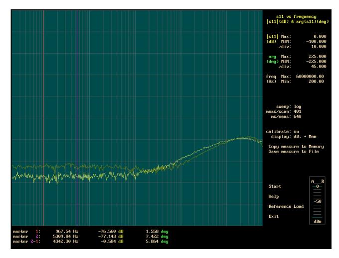
Impedance measurement of the A and R outputs (in the s11 format)
