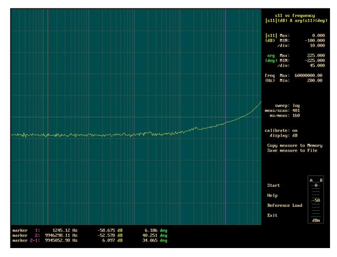
Impedance measurement of the (A) or (R) outputs (in the s11 format)
