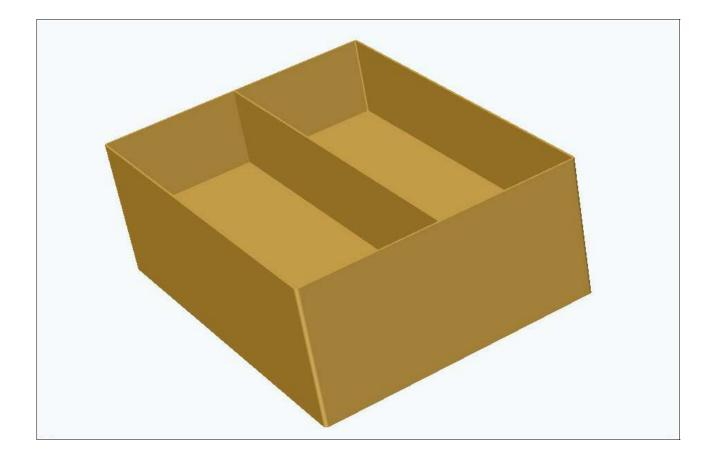
The outer wall of the box is made with an iron sheet, dimensions 551mm\*60mm\*0.8mm There is a bend in each corner.
