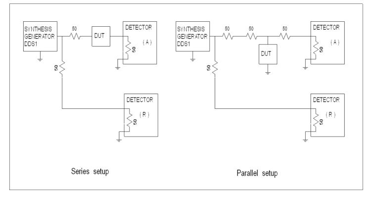
We can put the DUT in **series** between the generator (DDS1) and the input of the detector (A).
