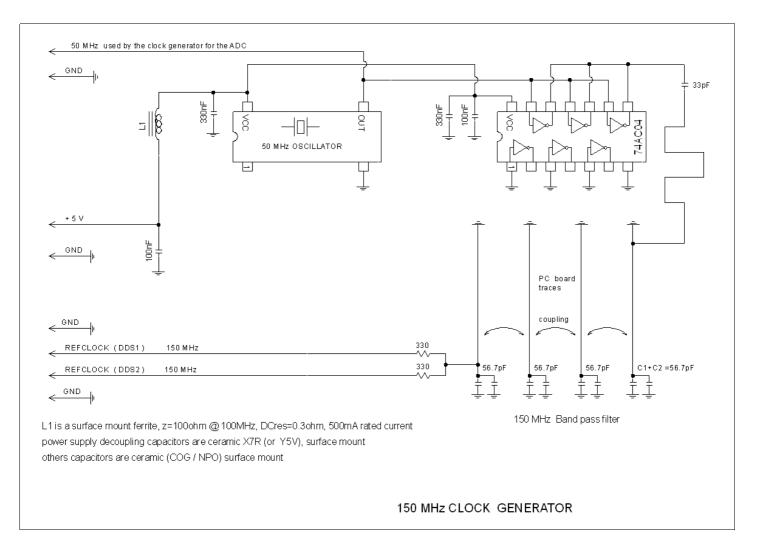
The AD9851 DDS generators need a clock at the frequency of 150 MHz.
