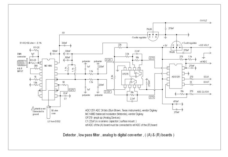
A balanced modulator (MC1496), mixes the input signal (A or R) with the local oscillator signal. At the output of the modulator, a low-pass filter removes the high frequencies content, to keep only the 25 Hz signal. For this filter, 1  $\mu$ F and 220 nF are polyester capacitors, ceramic capacitors (X7R or Y5V) vary too much with the temperature.
