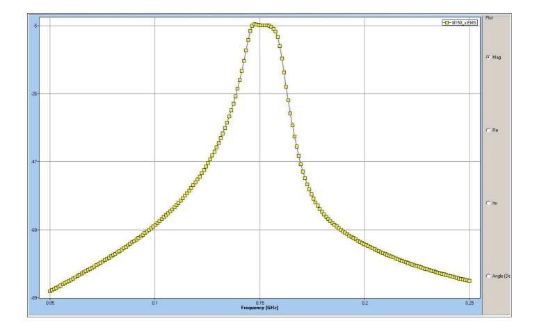
Frequency response of the 150 MHz filter (dB), (simulation).
